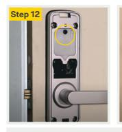
If not, press the internal button to switch between lock and unlock mode then try again. To complete the installation, replace the battery cover top end first and push in and up to lock into place. Your lock will turn on, ready to connect to your phone.
