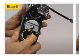
To hand the lock, hold down on the metal slide tab and rotate the handle left or right depending on your selected handing. Ensure you hold down the tab at all times during the rotation. Rotation should be smooth, if you experience firm resistance, release the handle and slide tab and repeat handing process. Ensure you complete this for both handles.
