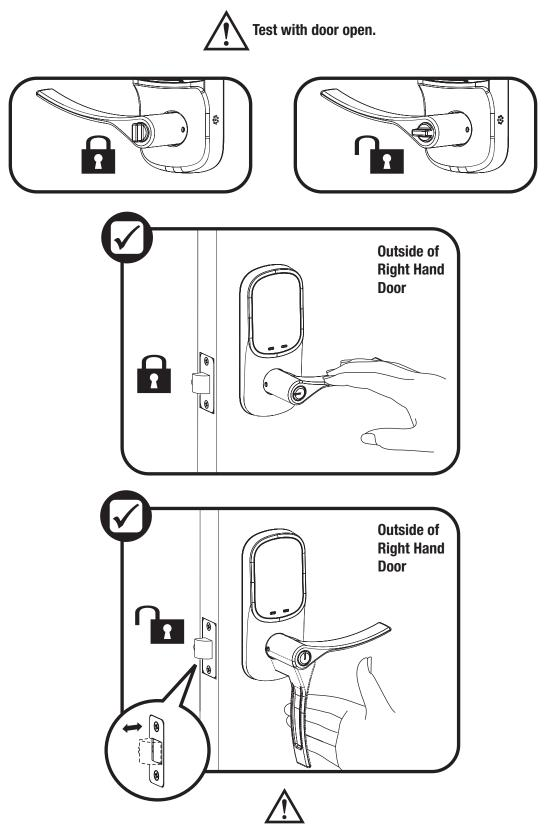
Test thumbturn and both levers in locked and unlocked positions. If operation fails, check installation beginning with Step 2 and refer to Hardware Troubleshooting.
