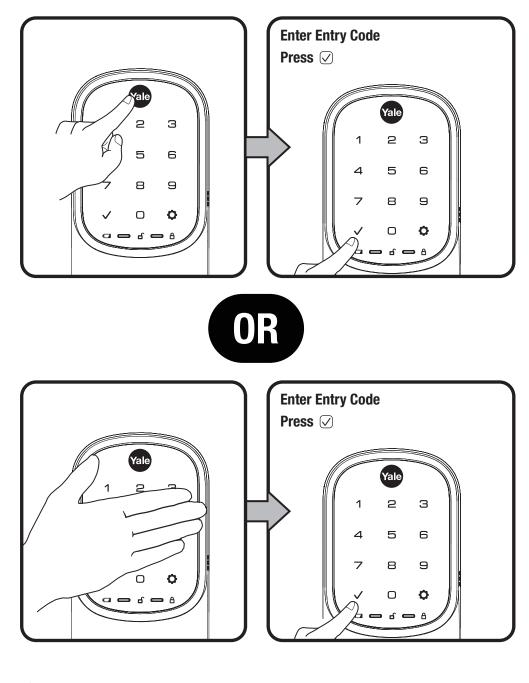
If touchscreen operation test fails, check installation beginning with Step 2.
