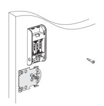
Fix screw to completely secure battery pack.
