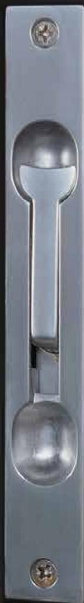
The Interlock flush bolt range is used for the safe bolting of aluminium doors and windows. The 7mm diameter plated steel rod provides high security and is activated by a strongly constructed die-cast zinc body and operating lever with comfortable finger grip.
