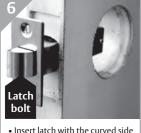
of the latch bolt facing in the direction that the door closes.
