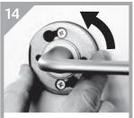
• Rotate rose furniture to align screws with countersunk holes
