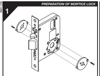
Attach adaptor plates to Lockwood 3570 mortice lock with screws provided
