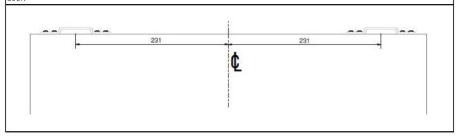
STEP 2: Route the bottom of the door, using the details shown
