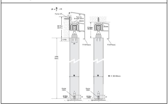
**STEP 5:** If face fixing the system, insert the fixing brackets into the top of the track. Then, using the edge of the opening as the centre point of the track, fix the track at the height identified in step 4.
