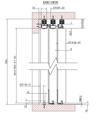
DT = DOOR THICKINESS DH = DOOR HEIGHT X = PCH RECOMMENDED TOP CLEARANCE (63,5MM) TSH = TRACK SET HEIGHT S = GAP REQUIRED BETWEEN TRACKS
