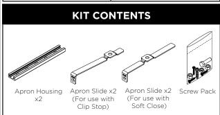
**NOTE:** APRON HOUSING REPLACES APRON PLATE INSTALLATION STEPS. (COMPATIBLE WITH HUSKY 120 PRO AND SOLTAIRE 120 SLIDING DOOR HARDWARE)
