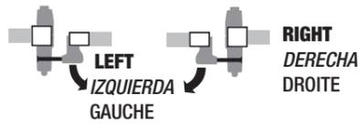
Rotate (flip) Mounting Bracket (A) to obtain the required Left or Right handing
