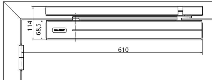
Space required on doors for standard installation on hinge side
