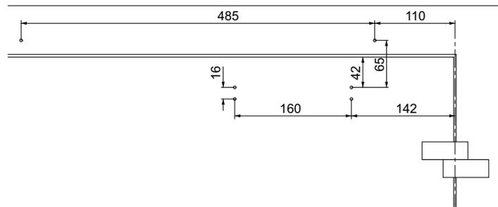
Installation dimensions for direct standard mounting on hinge side
