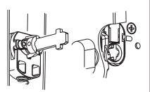
2. Engage tailbar end into the turn snib adapter as shown.
